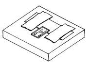
6. Place the acetate folder over the gage carrier, aligning sealed edge with top of gage endloops. Press lightly on the acetate folder and loosen the end of the gage carrier from tape mastic with a pair of tweezers.
