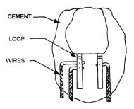
2. Fold the lead ribbons over the top of wires. Place a thin strip of copper under the ribbons.
