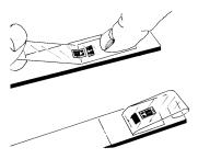
Lift one end of the tape at a shallow angle to surface (about 45 degrees) until gage and terminal are free of specimen surface. Tuck the loose end of the tape under and press to the surface so the gage lies flat with the bonding side exposed. In some cases this may be difficult
