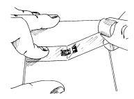
**Note:** Micro-Measurements PCT gage installation tape must be used if tape is employed to position the gage. Other tapes may react with uncured adhesive.
