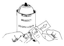
The surface preparation technique used is the same basic cleaning procedure described in Micro-Measurements Instruction Bulletin B-129, "Surface Preparation for Strain Gage Bonding". The initial step is to thoroughly degrease with solvents such as CSM Degreaser or GC-6 Isopropyl Alcohol. CSM Degreaser is preferred whenever possible since this is a very active degreaser. The substitution of GC-6 as a degreasing agent should be considered for materials that may be sensitive to strong solvents.
