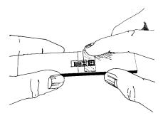
Remove the gage/tape/terminal assembly by peeling the tape at a shallow angle (about 30°) and transferring it onto the specimen. Make sure gage alignment marks coincide with specimen layout lines. If misalignment does occur, lift end of tape at shallow angle until assembly is free. Realign and replace. Use of a pair of tweezers often facilitates this handling.
