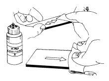
Dry-abrade the gaging area with 220- or 320-grit siliconcarbide paper to remove any scale or oxides on the base material. Apply M-Prep Conditioner A and wet-abrade the gage area. Keep the surface wet while abrading. Remove the residue and Conditioner by slowly wiping through the gaging area with a gauze sponge. The wet-abrade and wiping procedure should then be repeated with 400-grit silicon-carbide paper.
