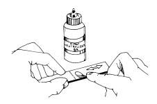
Apply a liberal amount of M-Prep Neutralizer 5A to the gage area. Keeping the surface wet, scrub with cotton-tipped applicators. Do not allow evaporation of the cleaning material on the specimen surface since this would leave a thin, unwanted film between the adhesive and the specimen.
