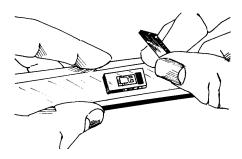
Place a silicone gum pad and backup plate (GT-14) over the gage installation. The silicone gum should be soft (Durometer A40-60) and at least 3/32 in (2.5 mm) thick. This will allow the clamping force to be exerted evenly over the gage. The area of the silicone gum pad should be used to compute the final clamping pressure.
