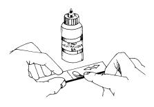
Apply a liberal amount of M-Prep Neutralizer 5A to the gage area. Keeping the surface wet, scrub with cotton-tipped applicators. Do not allow evaporation of the cleaning material on the specimen surface since this would leave a thin, unwanted film between the adhesive and the specimen.
