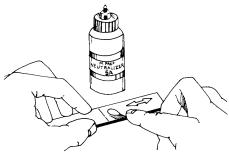
Apply a liberal amount of M-Prep Neutralizer 5A to the gage area. Keeping the surface wet, scrub with cotton-tipped applicators. Do not allow evaporation of the cleaning material on the specimen surface since this would leave a thin, unwanted film between the adhesive
