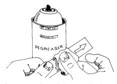
The surface preparation technique used is the same basic cleaning procedure described in Micro-Measurements Instruction Bulletin B-129, "Surface Preparation for Strain Gage Bonding". The initial step is to thoroughly degrease with solvents such as CSM Degreaser or GC-6 Isopropyl Alcohol. CSM Degreaser is preferred whenever possible since this is a very active degreaser. The substitution of GC-6 as a degreasing agent should be considered for materials that may be sensitive to strong solvents.
