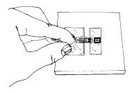
Remove a gage from its mylar envelope with tweezers, making certain not to touch any exposed foil. Place the gage, bonding side down, onto a chemically clean glass plate or empty gage box. If a solder terminal is to be incorporated, position it next to the gage. While holding the gage in position with a mylar envelope, place a short length of MJG-2 mylar tape down over about half of the gage tabs and the entire terminals.
