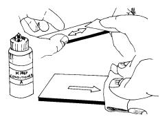
Dry-abrade the gaging area with 220- or 320-grit siliconcarbide paper to remove any scale or oxides on the base material. Apply M-Prep Conditioner A and wet-abrade the gage area. Keep the surface wet while abrading. Remove the residue and Conditioner by slowly wiping through the gaging area with a gauze sponge. The wet-abrade and wiping procedure should then be repeated with 400-grit silicon-carbide paper.
