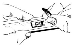
Overlay the gage/terminal area with a piece of thin Teflon sheet (TFE-1). If necessary, anchor the Teflon in place with a piece of Mylar tape across the end. Place a silicone gum pad and backup plate (GT- 14) over the gage installation. The silicone gum should be soft (Durometer A40-60) and at least 3/32 in (2.5 mm) thick. This will allow the clamping force to be exerted evenly over the gage. The area of the silicone gum pad should be used to compute the final clamping pressure.
