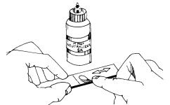
Apply a liberal amount of M-Prep Neutralizer 5A to the gage area. Keeping the surface wet, scrub with cotton-tipped applicators. Do not allow evaporation of the cleaning material on the specimen surface since this would leave a thin, unwanted film between the adhesive
