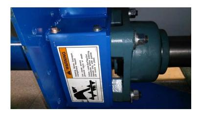
B: Strain gage area with its protective cover
