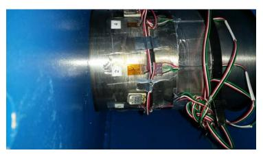
Picture 5: Strain gages installed on the reclaimer screw shaft: two full-bridges in shear patterns (torque) and two half-bridges in linear patterns (bending)
