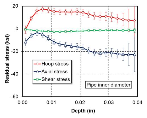
Figure 2: Residual stress measurement data from hole drilling at the inner diameter of a welded pipe
