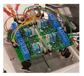
Figure 1: Student made amplifiers on suspended mounting for shock absorption and vibrations.
