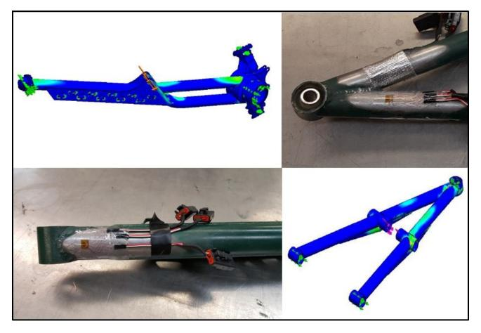
Figure 2: FEA model of trailing arm (top left). Stacked rosette applied to trailing arm (bottom left). Lower Aarm with a stacked rosette applied to each side with one covered by thermal reflecting tape (top right). FEA model of lower A-arm (bottom right).
