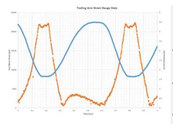
Figure 4: Trailing arm data. (Blue curve) Linear potentiometer linear displacement of distance versus time [in v. sec] (Orange curve) Von Misses stress from strain gage rosette versus time [psi v. sec].
