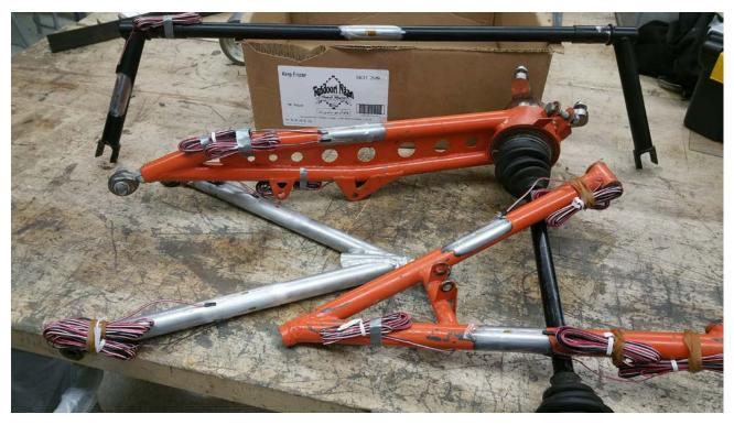
Figure 1: Gaged and Calibrated Suspension Components Ready for Testing
