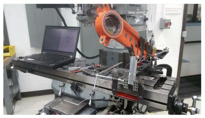
Figure 2: Trailing Link Calibration by Hanging Calibrated Weight Sets NOTE: Calibration with ANSYS was verified by limited calibrated weight set testing and then used to further apply loads in order to fully cover expected loading ranges.
