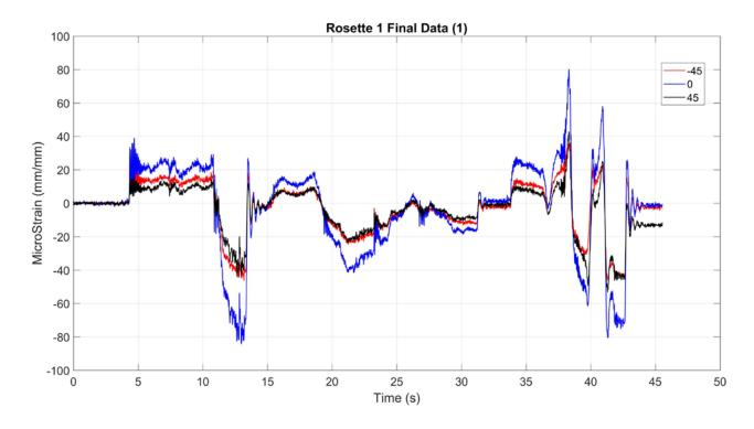
Figure 1: Sample data from one rosette through dynamic testing
