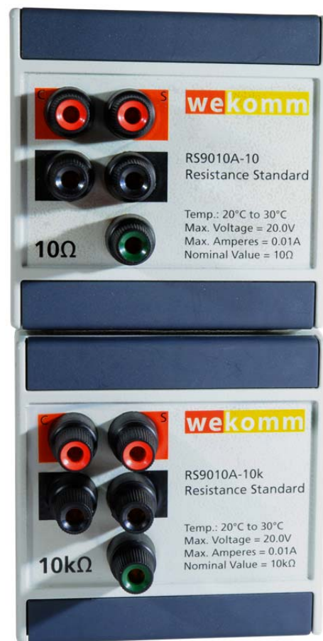
Figure 1: wekomm engineering's 10 Ω and 10 kΩ precision resistance standards pair the VFR VHA518-7 Bulk Metal Foil resistor with carefully selected components to form a transfer standard product housed in a protective aluminum case.
