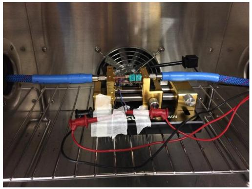
Fig.4 — Inside of the temperature chamber
