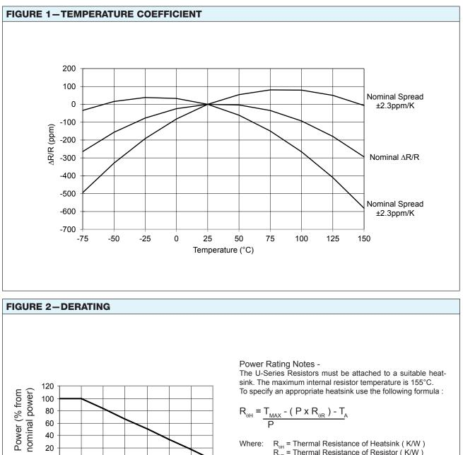
$$R_{\theta H} = \frac{T_{MAX} - (P \times R_{\theta R}) - T_{A}}{P}$$
