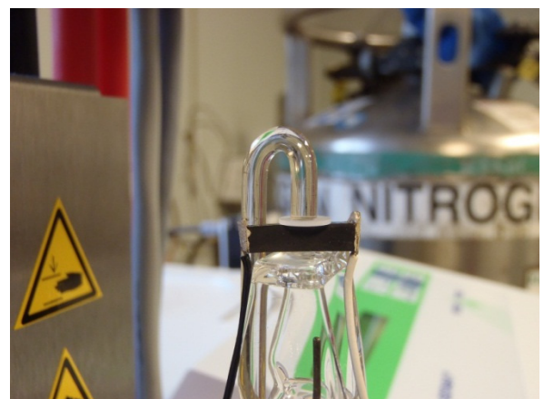
Fig 1: Image of a specimen mounted on a thermomechanical analyzer stage.
