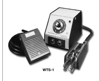
The ease and simplicity of operation of the Thermal Wire Stripper make it ideal for most strain gage leadwire stripping. The variable heat control allows stripping of all thermoplastic insulations, including Teflon®, in sizes No. 18 to No. 36 AWG (1 to 0.1 mm diameter). The foot switch and tweezer handspiece give excellent operator control over the stripping operation. Includes power unit and foot switch, both with 3-wire NEMA plugs, and tweezer handpiece.
