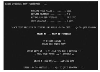
Figure 3. STO for thin film resistor
