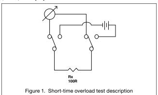
The test measures the change in resistance of the subject resistor due to the applied overload. The screen displays the  $\Delta R/R$ , which is the variation of the resistance readings taken before and after the overload.
