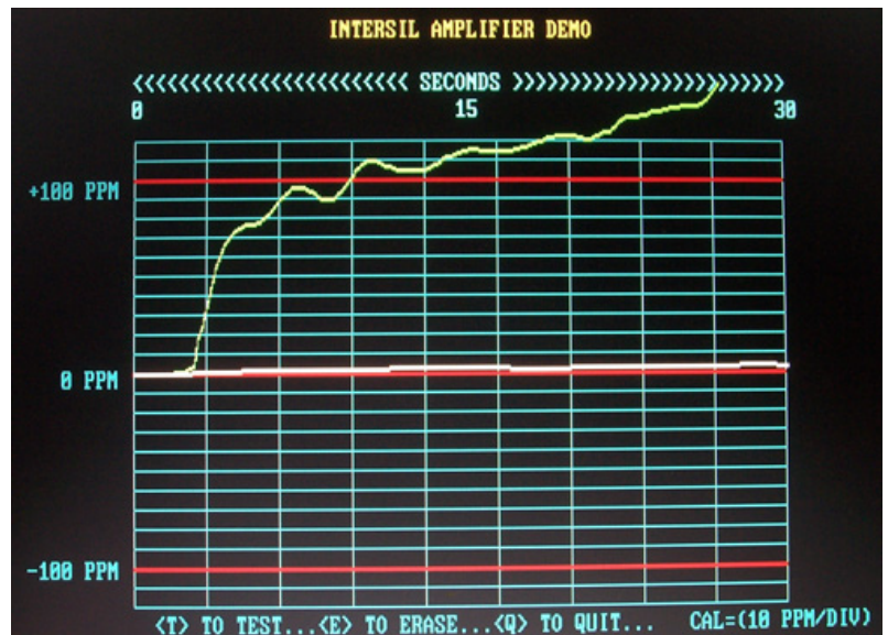
Figure 4 – Graph showing the resistance change in ppm from initial value of the resistors (R1 and R2) due to the rise of the ambient change caused by the heat gun
