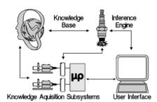
The LCp-104 uses the expert system concept to compare various measurements against known standards of acceptable performance and uses that relative comparison to identify and diagnose both transducer and system performance problems. The BLH expert system identifies piping influences, structural problems, transducer drift, cell overload, and the location and characteristics of process noise.
