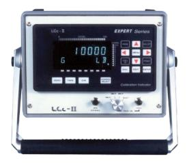
Hot key displays provide instant access to cell mV/V output, peak, valley, zero, and tare values. To check calibration, three standard values are switch selectable along with a fourth provision for a user supplied resistor. Rear panel tension or compression selection reverses polarity if needed. Signal communication is available in 16 bit analog output and RS-422/485 digital formats. The RS-422 signal can be used for printouts or a full, bi-directional PC interface.
