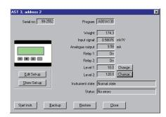
and printed deltaCOM displays live weight and status information and provides a work area to enter and change various weigh system parameters. The status of the set-up can be checked also during operation.
