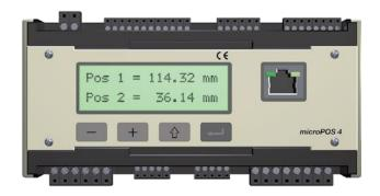
compared to feedback values, measured by position transducers or load cells. Parameters in the servo unit are used to control maximum speed, acceleration, and working range for the servo channels.
