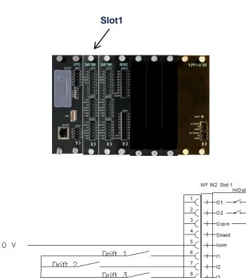
For the separate channels, any of the other inputs can be configured to accumulate time and calculate full load hours for resp. channel.
