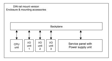
Block structure of a G4 Instrument
