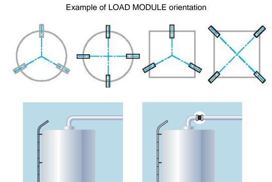
To achieve good weighing results, always use flexible connections to the vessel and check that no ladders or other arrangements connect the weighed vessel to surrounding foundation, walls or roof.
