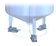
Check again the measure "**x**" between BRACKET and YOKE, and that the lateral play between YOKE and LOAD CELL is preserved. See point 3 and 4.
