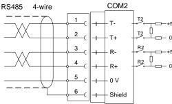
The communication lines must be terminated in both ends. If G4 is connected at the end of the communication line switches must be set as:
