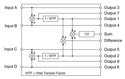
Four Channel Function block, Web Tension mode
