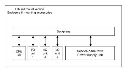
Block structure of a G4 Instrument
