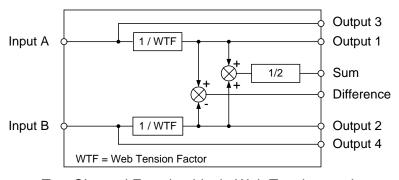
Two Channel Function block, Web Tension mode
