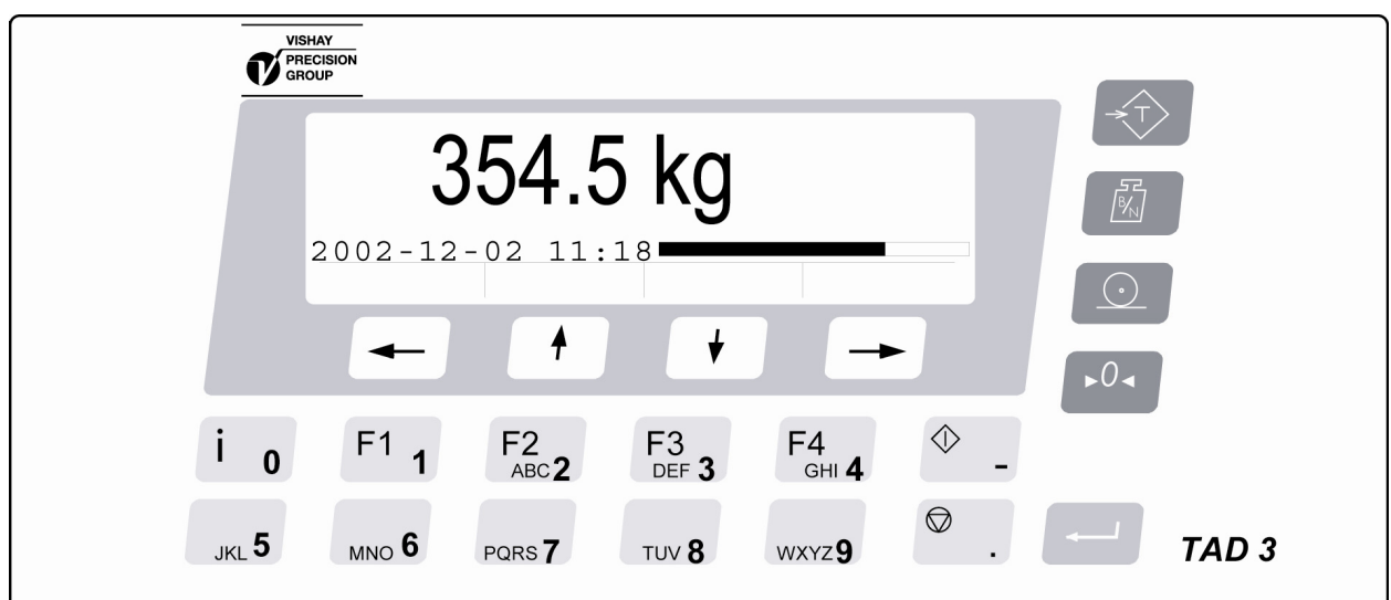
Figure 7. Front panel of TAD 3 with LCD-display, four function keys below the display, four keys with weighing symbols to the right, twelve keys with digits and letters, and an ENTER key.
