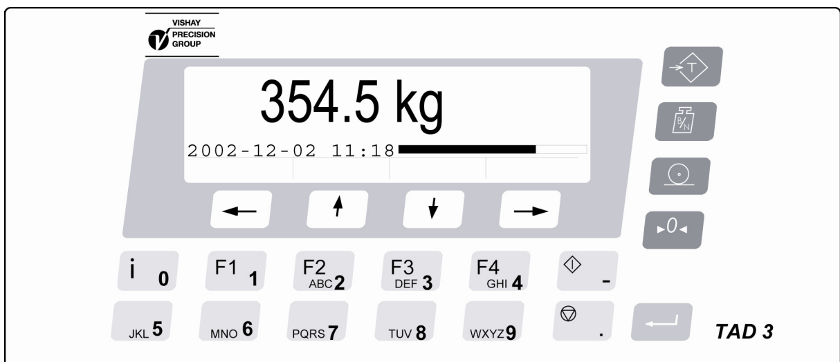
Figure 11. TAD 3 front panel by normal weighing operation.
