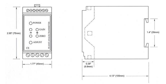
Figure 2. PS1010T Mechanical Dimensions.
