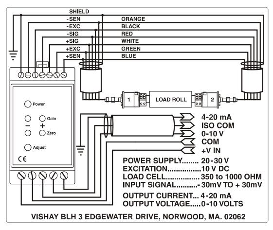
Figure 1. PS1010T Electrical Wiring.
