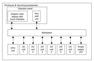
Block structure of a G4 Instrument
