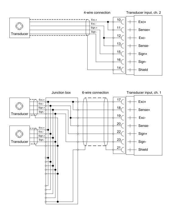
A transducer may be connected directly to terminals at the transducer input. For several transducers or long distance, a junction box and lengthening cable is needed. For a HS WF2 channel, the shield can be connected to ground/earth at any point
