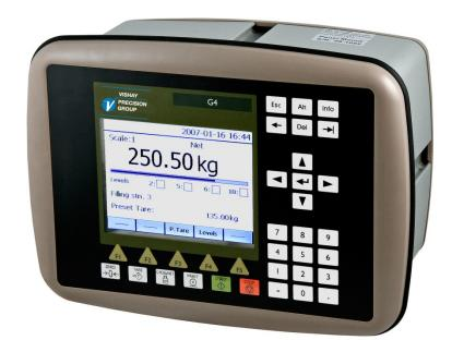
Front panel of the G4 instrument with color touch display, five function keys below the display, six application specific keys, numerical keypad, joystick keypad (arrow keys), Esc, Alt, Backspace, Delete, Tab and ENTER keys. In addition there is an Info key that is used to access the instruments menu system.
