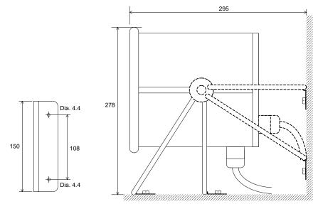
DT and HE instruments. Fixing bracket, recommended distances to surrounding surfaces.
