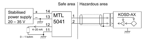
Load cell KIMD-AX with 100 m of integrated cable, used in a hazardous area. The load cell cable is connected by diode safety barriers, where the cable shield is not to be connected to ground. The load cell cable parts can be connected to any polarity.
