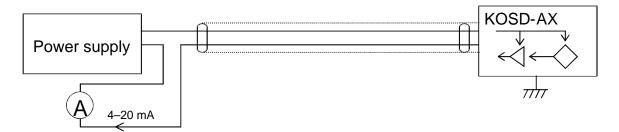
Load cell KOSD-AX with a cable connector, used in a hazardous area. A shielded cable is connected to the load cell. An isolating IS unit is used. The load cell cable parts can be connected to any polarity.
