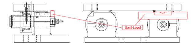
Depending on the application, the wrap angles and the nominal tension forces, the KIS load cells can be oriented either vertically or horizontally. In order to have the KIS load cells properly oriented, check the arrow direction. In order to perform this load cells orientation, use a spririt level to check horizontality or verticality the working direction of the KIS loadcell.
