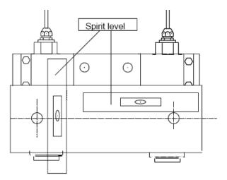
b) Check that the KIS/KISD load cells are properly fixed on their block supports (surface A on the KIS load cell should be on the same level as the surface B on the KIS mounting block. Thereafter check that the KIS/KISD load cells are properly orientated vertically, horizontally or in the direction of the resultant force FR, depending on the application. Normally this is already performed at delivery.
