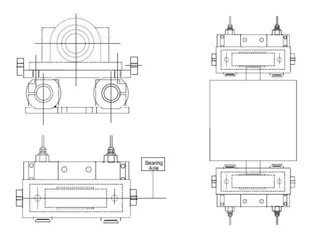
Adjusting the parallelism of the measurement roll relative to the other rollers of the machine. This can be done manually, or if requested at order, the FMU-1 and FMU-5 web tension unit can be delivered with screw adjustments on each side of the top plate, to simplify this operation.
