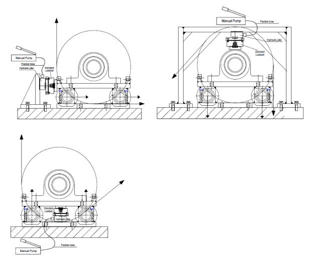
This method needs some investments at installation for the Hydraulic calibration system, but during maintenance calibration and checks do not need too much time at each calibration or check: About one hour per roller when everything goes all right.
