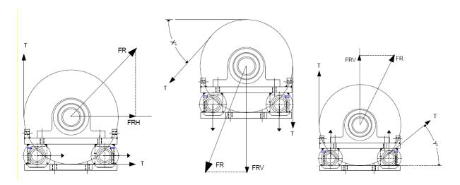
Then according to T Max and to the wrap angle  $X^\circ$  or  $Y^\circ$ , the resultant Force FR must be calculated as well as the Vertical Force FRV or the Horizontal Force FRH.
