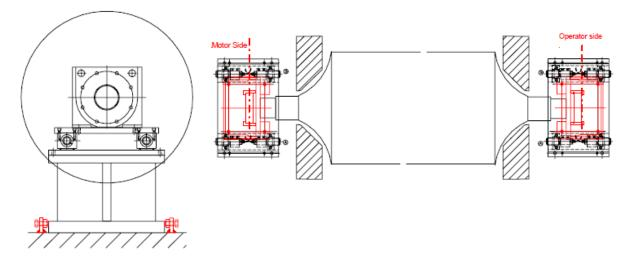
c) Setting of the bearings / web tension unit parallelism on the measuring roll.
