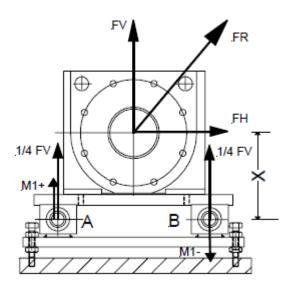
One of the others features of the KIS loadcells is that the signal outputs of the loadcells are matched to 2,04 mV/V + 0,1 %, which means that if M1+ and M1- are identical in force, they are also identicals in term of electrical outputs.
