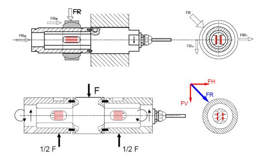
The resultant force FR on the roller or on the KIS load cell will consist of three basic forces:
