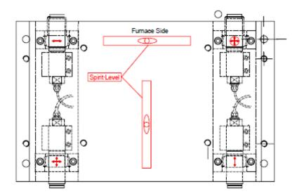
b) Check that the KIS load cells are properly fixed on their block supports (Surface A on the KIS load cell should be on the same level than surface B on the KIS mounting block), and properly oriented (Arrow / KIS load cell oriented vertically or horizontally, depending on the application). See drawing below.
