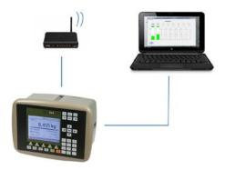
Figure 1: G4 with remote display on PC
