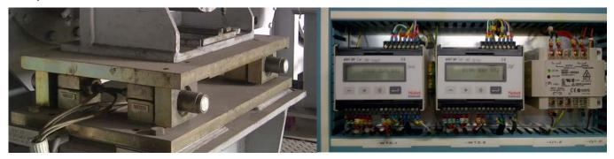
Figure 3: A PST web tension unit installed in a web tension measuring station, including the corresponding measuring amplifier
