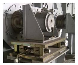
Figure 1: PST web tension measuring unit
