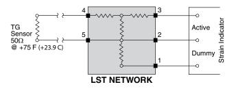
To optimize performance, separate network designs are available for select temperature ranges covering cyrogenic to +500°F. The environmental temperature range for LST networks is  $-65^{\circ}$  to +250°F (-55° to +125°C). Standard strain gage instrumentation, such as the Micro-Measurements Model P3, is ideal for use with these sensors, eliminating the need to purchase separate readout devices.
