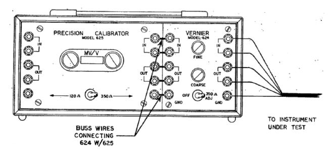
Figure 2-7. Combination Model 624/625 Connections
