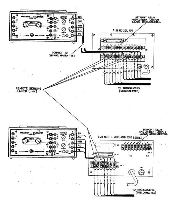
Figure 2-8. Typical 624 Connections to BLH Equipment
