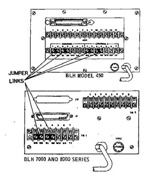
Figure 2-6. Jumper Links Installed.
