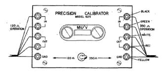
Figure 2-1. Model 625 Connections.
