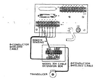
Figure 2-5, Remote Sensing Connections.
