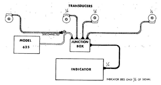
Figure 3-2. Four Transducer System Calibration.
