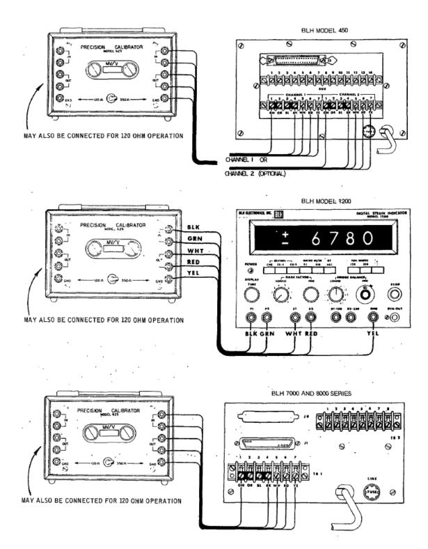
Figure 2-2. Typical Connections to Various BLH Equipment
