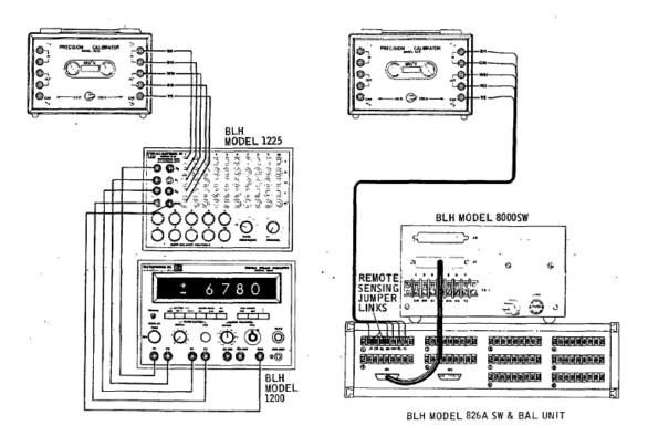
Figure 2-4. 625 Used with Switching and Balancing Units
