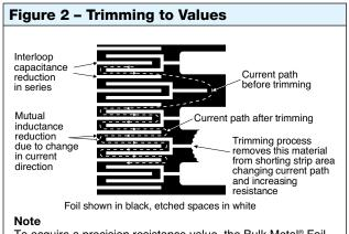
To acquire a precision resistance value, the Bulk Metal® Foil chip is trimmed by selectively removing built-in "shorting bars." To increase the resistance in known increments, marked areas are cut, producing progressively smaller increases in resistance. This method reduces the effect of "hot spots" and improves the long-term stability of Bulk Metal® Foil resistors.
