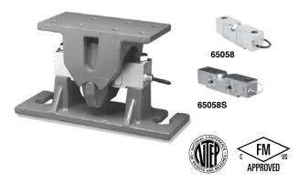
This product is designed to simplify the installation of the 65058 load cell into a certified Legal-for-Trade high capacity weigh bridge. Unilink  $^{\text{TM}}$  floating suspension allows controlled floating of the scale deck, providing a reliable and accurate weighing system. The load cell is nickel plated or stainless steel and sealed to IP67 standards, assuring reliability. The mount assembly is provided with a primer coat finish to simplify the manufacture of the scale.
