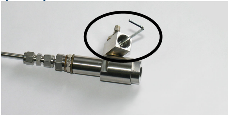
Figure 2. Removing the leak screw
