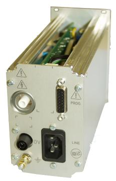
$\underline{\text{OUTPUT ISOLATION:}}$  The "0V" - terminal of the output is connected to earth on the back panel and may be disconnected as needed. When disconnected, the "0V" terminal may float with respect to earth up to  $\pm 125$  V.
