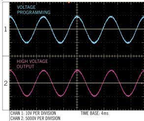
Figure A: 5HVA24-BP1 Sine Wave Input
