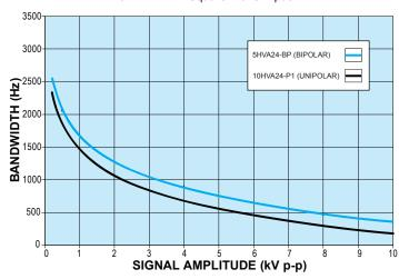
Figure F: Bandwidth vs. Signal Amplitude with 100pF Load
