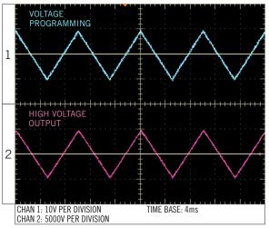
Figure C: 5HVA24-BP1 Triangle Wave Input
