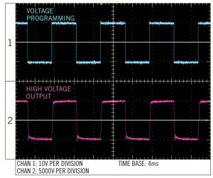
Figure D: 5HVA24-BP1 Square Wave Input
