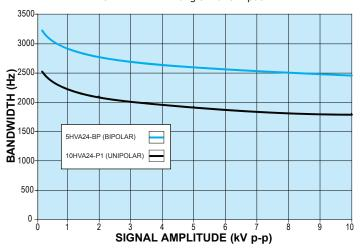
Figure E: Bandwidth vs. Signal Amplitude with No Load
