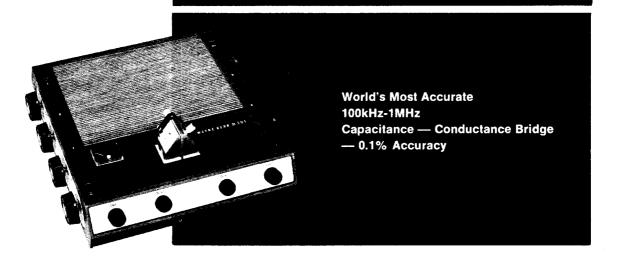
Designed for highly precise, simultaneous in-circuit measurement of capacitance and conductance over an extremely wide range — from 0.001pF-10.000pF and from 0.01 $\mu$ MHo-100Mho — the B201 Bridge is invaluable for checking capacitors and components of printed circuits and/or encapsulated assemblies. The extremely wide measurement range is covered by the combined use of a 3-position multiplier switch, alternative connections for the Unknown, and optional Low Admittance Adaptor.
