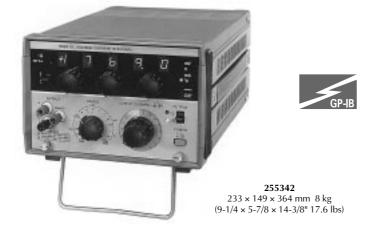
The 2553 is an ultra-stable, high-resolution DC voltage and current source which delivers output voltages from 1  $\mu$ V to 12 V, and output currents from 0.1  $\mu$ A to 120 mA at an accuracy of ±0.02%.
