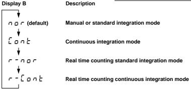
After the desired integration mode has been selected, press the ENTER key.
