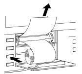
5. Push the middle of the guide in the direction shown by the arrow to secure the paper.
