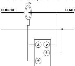
When Voltage is Output from the External Sensor
