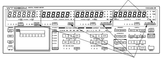
The specific type of information to be displayed is shifted downwards each time the *FUNCTION* key is pressed.
