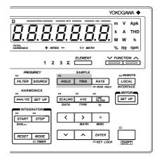
If the measured values are output (by means of a communications channel or the D/A converter), the output values are also updated when the  $\mathsf{TRIG}$  key is pressed.
