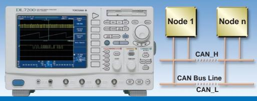
Evaluating the physical layer in the Controller Area Network (CAN) bus widely used for automotive applications is essential to analyzing communication failures that may occur, in particular, for such reasons as noise resulting from surge voltages or level fluctuations resulting from post-wiring overloads. The CAN BUS SIGNAL ANA-LYZER captures and analyzes the waveforms of bus signals that proved difficult with conventional protocol analyzers alone.
