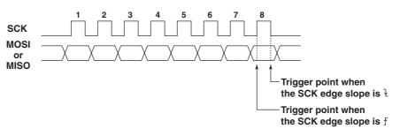
This section will indicate the data sequence at the byte level in hexadecimal and indicate the position where the trigger will occur.
