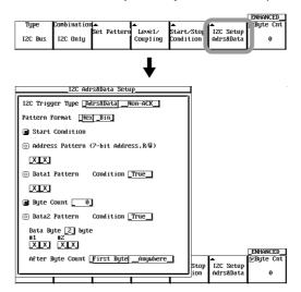
To activate triggers on the start condition or address pattern/data pattern, proceed to step 5 below. To activate triggers when an Acknowledge bit is not detected (Non-Ack trigger), proceed to step 16 on the next page.
