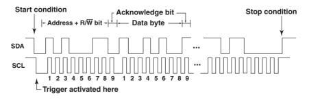
When Activating a Trigger on the Address Pattern/Data Pattern
