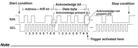
The Acknowledge bit of the start byte and Hs mode master code is not applicable.
