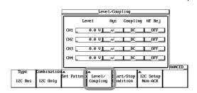
31. Press ESC. The Level/Coupling dialog box closes.
