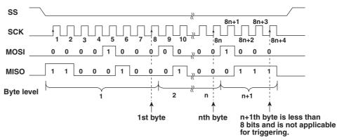
To activate triggers on the DL1740E/DL1740EL, you will set pattern A/B and/or byte count. Triggers can be activated in various ways such as when the MOSI data pattern matches pattern A; the specified byte count after the MOSI data pattern matches pattern A; or when the MISO data pattern matches pattern B after the specified byte count elapses after the MOSI data pattern matches pattern A.
