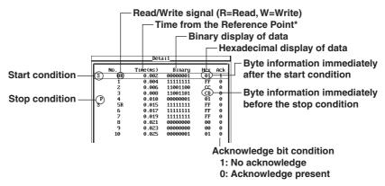
On the detailed display screen, the data corresponding to the specified number are highlighted.
