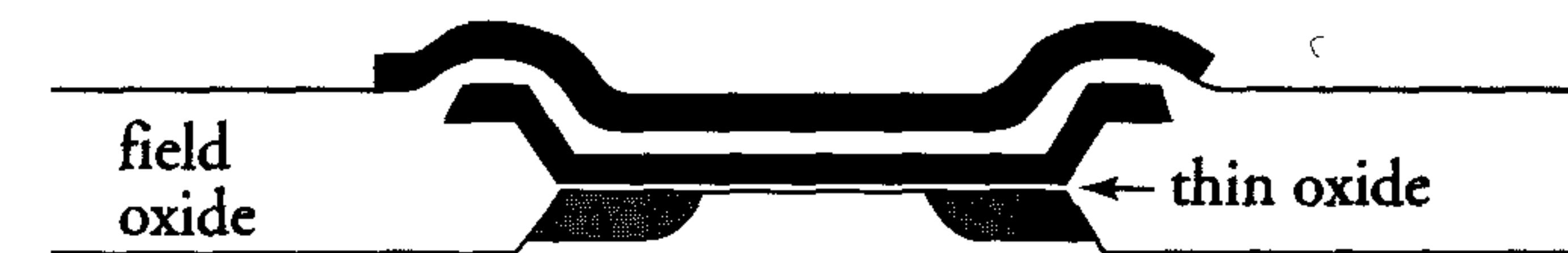
Figure 6.19: Cross-section of a flash EEPROM
