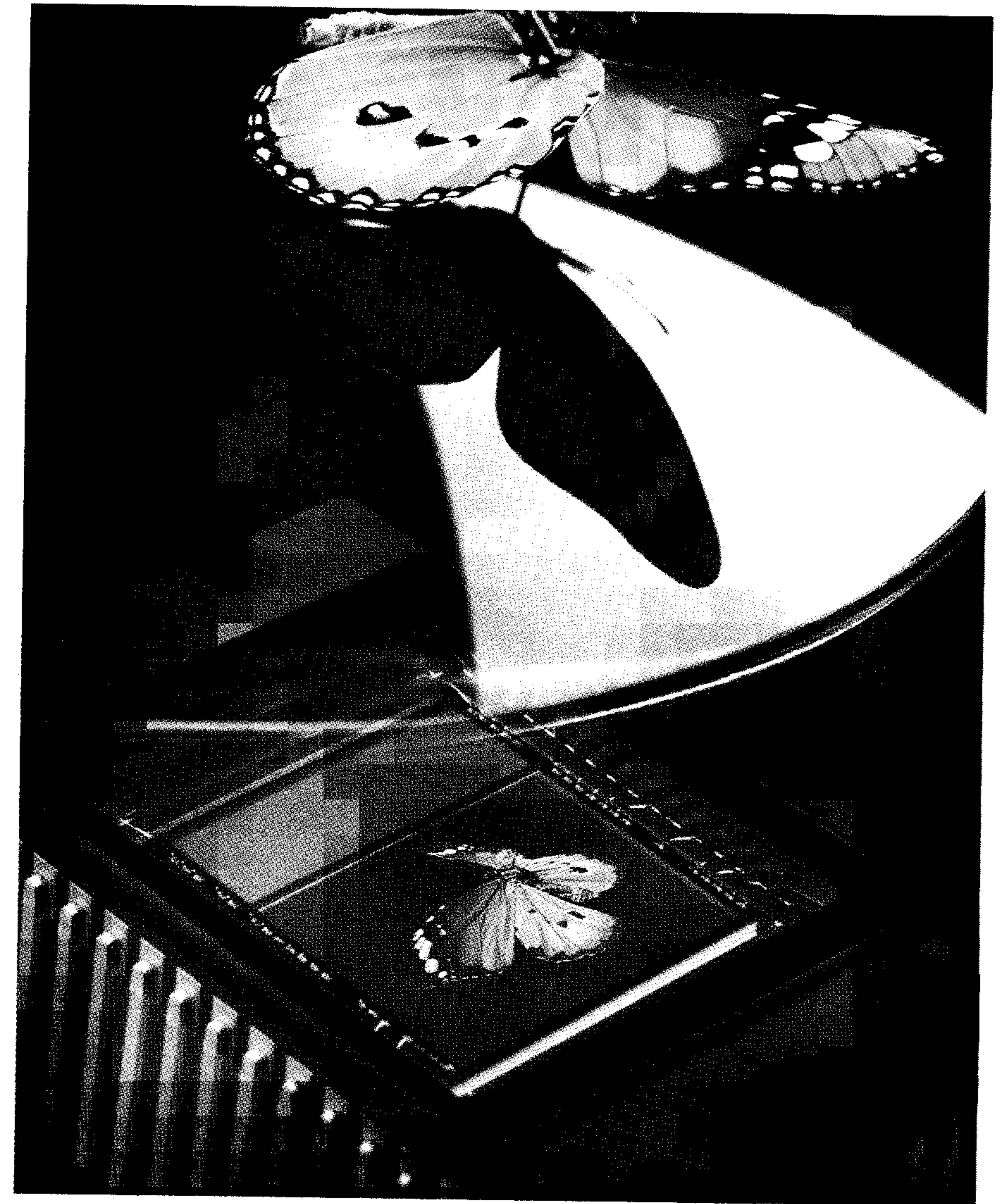
Figure 5.4: A CCD image sensor (photo: PHILIPS)
