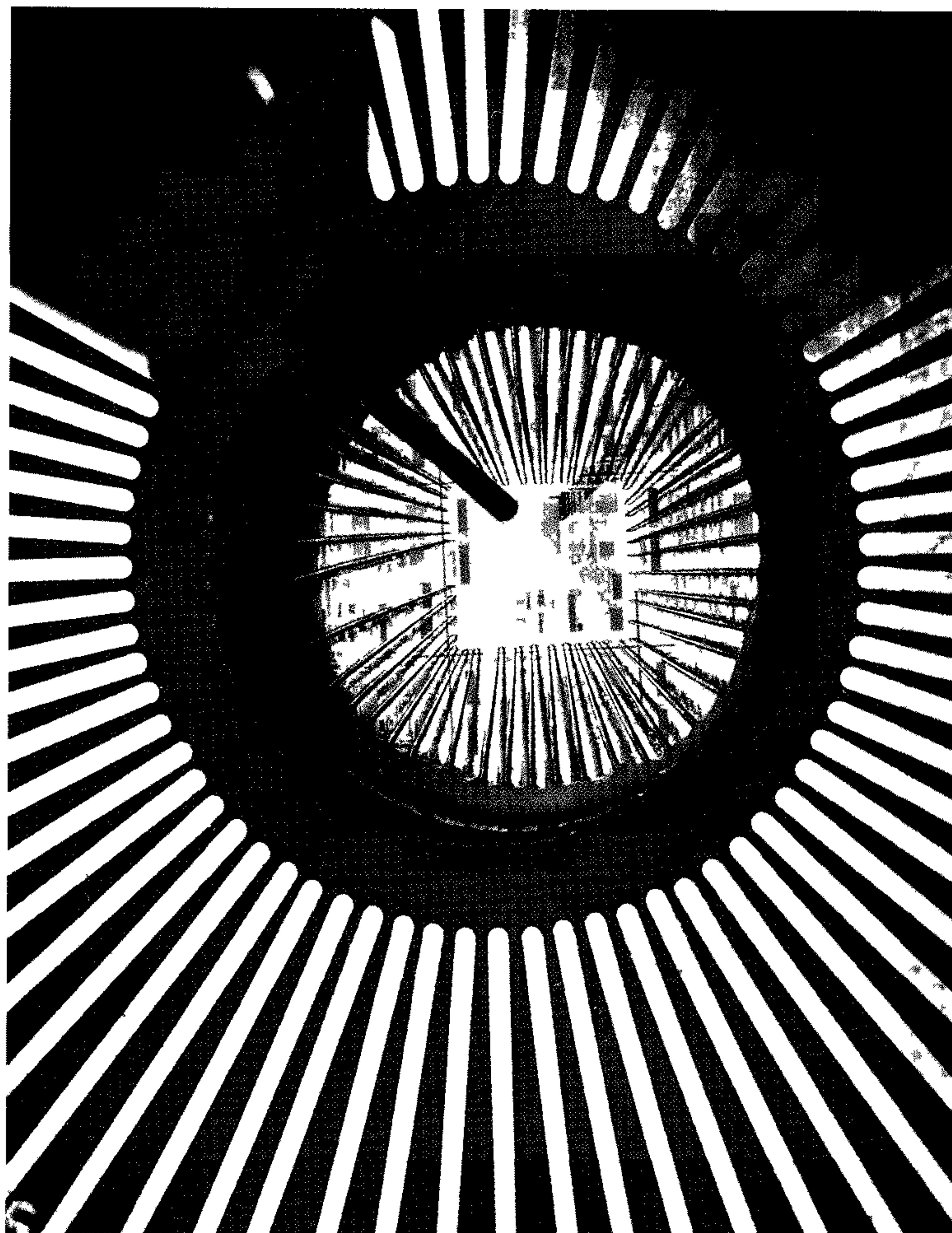
Figure 10.1: Probe card with probes and a chip in a test environment (Photo: PHILIPS)
