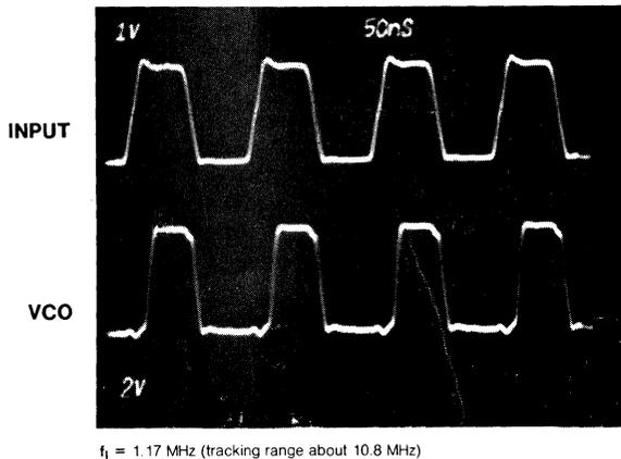
$f_L = 1.17 \text{ MHz}$  (tracking range about 10.8 MHz)
