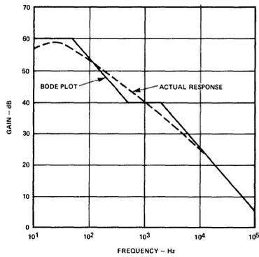
Bode Plot of RIAA Equalization and the response realized in an actual circuit using the 531.
