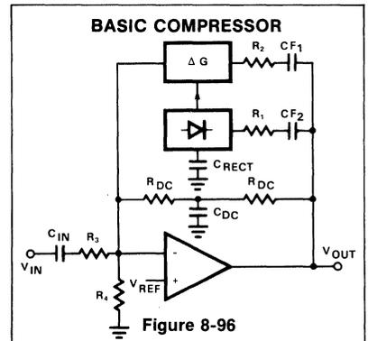
The same restrictions for the rectifier and ΔG cell maximum input current still hold, which place a limit on the maximum compressor output. As in the expander, the rectifier and ΔG cell inputs could be made common to save a capacitor, but low level tracking accuracy would suffer. Since there is no dc feedback path around the op amp through the ΔG cell, one must be provided
