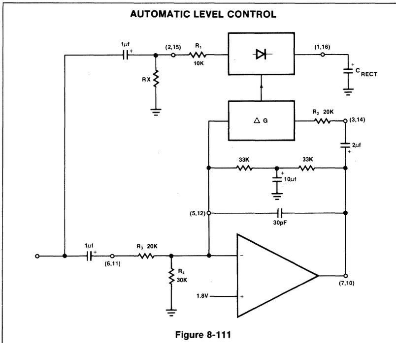
tion ratio is desired, proper selection of fixed resistors can be used instead of the potentiometer. The optional threshold resistor will make the compression or expansion ratio deviate towards 1:1 at low levels. A wide variety of (input) output characteristics can be created with this circuit, some of which are shown in Figure 8-113.
