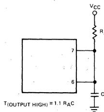
$T_{(OUTPUT HIGH)} = 1.1 R_A C$
