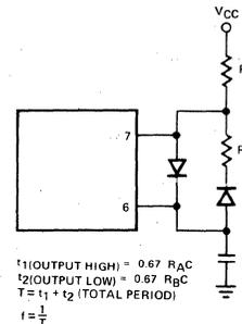
$t_1(OUTPUT HIGH) = 0.67 R_A C$
