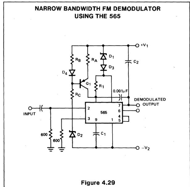
rent can be varied only a small amount due to the small change in current through  $R_1$ . Consequently, the VCO can track the input signal over a small frequency range yet the output voltage of the loop (control voltage of the VCO) will swing its maximum value.
