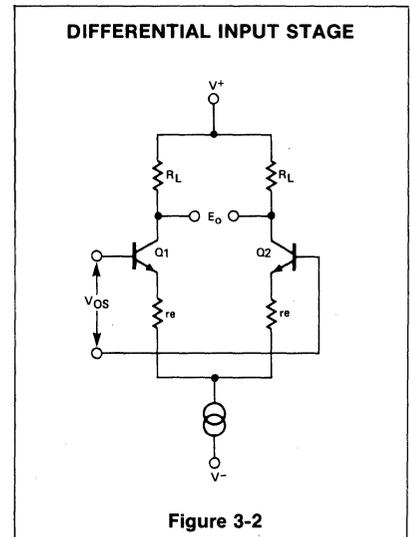
$$E_{OS} = I_{C2}R_L - I_{C1}R_L = 0 \quad (3-1)$$
