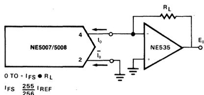
For complementary output (operation as negative logic DAC), connect inverting input of OP-amp to I<sub>o</sub> (pin 2), connect I<sub>o</sub> (pin 4) to ground.
