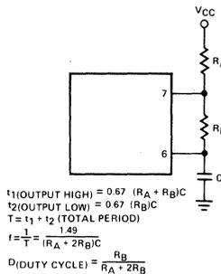
$t_1(OUTPUT HIGH) = 0.67 (R_A + R_B) C$
