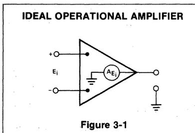
Further desirable attributes would include infinite bandwidth, zero offset voltage, and complete insensitivity to temperature, power supply variations, and common mode input signals.
