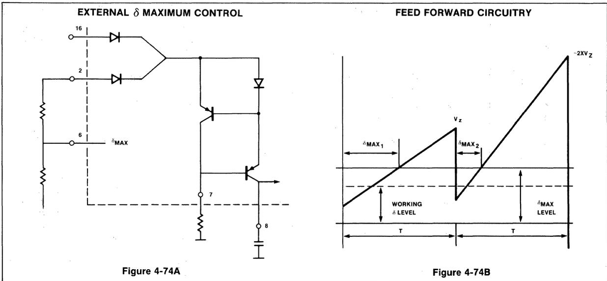
increases also. Note that the  $\delta_{max}$  voltage on pin 6 remains constant because it is set via  $V_z$ . Figure 4-74B visualizes the effect on  $\delta_{max}$  and the normal operating duty cycle  $\delta$ . For  $V_{16} = 2xV_z$  these duty cycles have halved. The graph for  $\delta = f(V_{16})$  is given in Figure 4-75.
