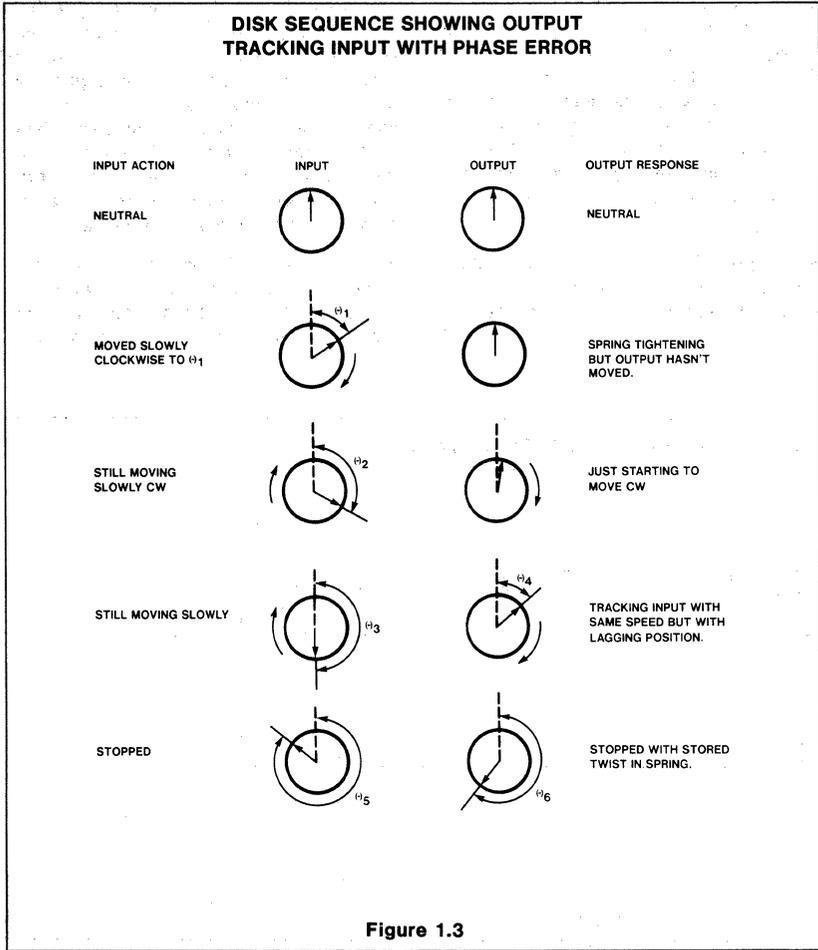
If the rate of the input disk is alternately increased and decreased by some small amount compared to the nominal revolution rate, the positional markers will appear to walk both clockwise and counter clockwise, momentarily appearing stationary when the strobing light rate equals the disk revolution rate. This "walking" represents a changing phase error which is occurring at the modulation rate. Thus the phase error can be thought of as a useable demodulated output signal.
