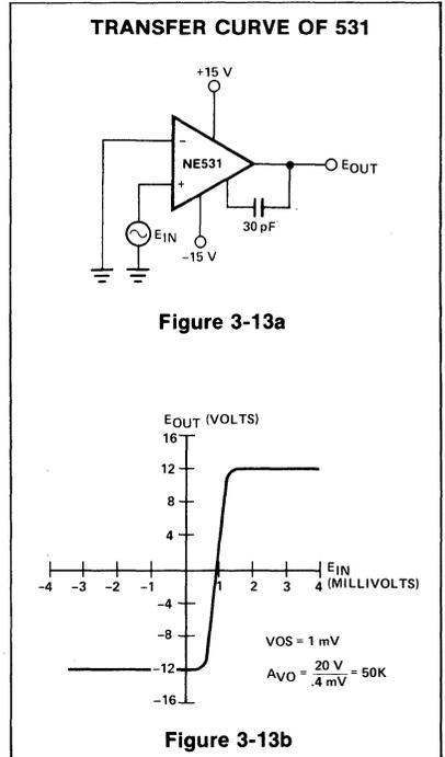
and +10 volts where it crosses the  $E_{in}$  axis, the voltage gain and offset voltage may be determined. It can be seen that the voltage gain of the device under test, (D.U.T.), is 50,000 and its input offset voltage is 1.0mV.
