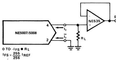
For complementary output (operation as a negative logic DAC), connect non-inverting input of OP-amp to I<sub>o</sub> (pin 2); connect I<sub>o</sub> (pin 4) to ground.
