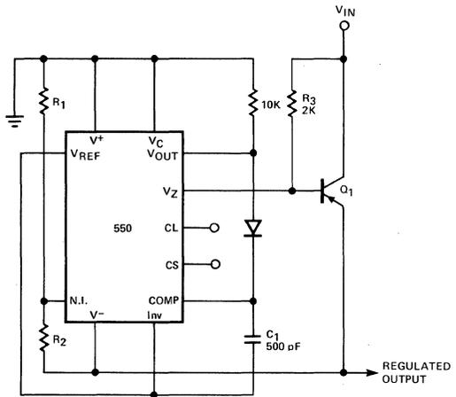
$$V_{OUT} = -V_{REF} \times \frac{R1 + R2}{R2}$$
