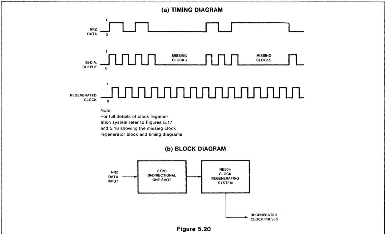
The circuit diagram for an NRZ system using the 564 is shown in Figure 5.21. Experimental waveshapes obtained with this system operating at a 1.0MHz data rate are shown in Figure 5.22. The 564 remained in lock for up to 15 missing clock pulses. The waveshapes show system operation for 4 and 8 missing clock pulses.
