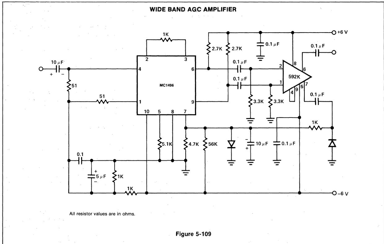
84, the signal is fed to the signal input of the MC1496 and RC coupled to the NE592. Unbalancing the carrier input of the MC1496 causes the signal to pass thru unattenuated. Rectifying and filtering one of the NE592 outputs produces a dc signal which is proportional to the ac signal amplitude. After filtering this control signal is applied to the MC1496 causing its gain to change.
