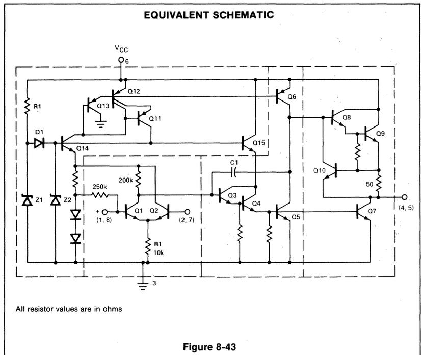
In applications where noise is less critical, Q1 and Q2 can be used in the differential configuration. This has the advantage of higher impedance at the feedback summing point, allowing the use of larger resistors and smaller capacitors in the one control and equalization networks.
