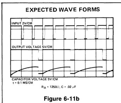
Figure 6-11b shows the waveforms of the timer in Figure 6-11a when used as a divide by three circuit. This application makes use of the fact that this circuit cannot be retriggered during the timing cycle.
