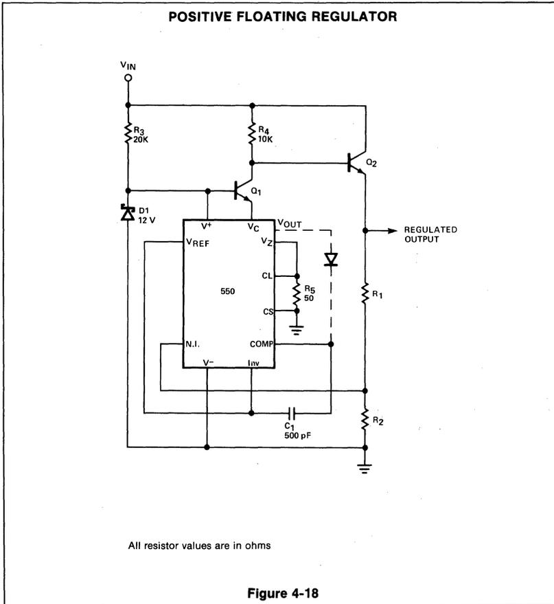
tion can be overcome by using floating regulator techniques.
