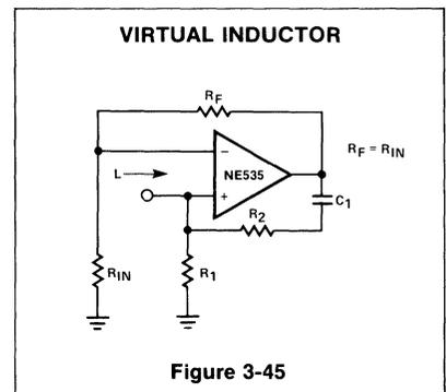
verses. The NE535 device will work up to 10kHz with less than 5% distortion.
