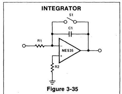
Since the gain at dc is very high a method for resetting initial conditions is necessary. Switch  $S_1$  removes the charge on the capacitor. A relay or FET may be used in the practical circuit. Bias and offset currents and offset voltage of the switch should be low in such an application.
