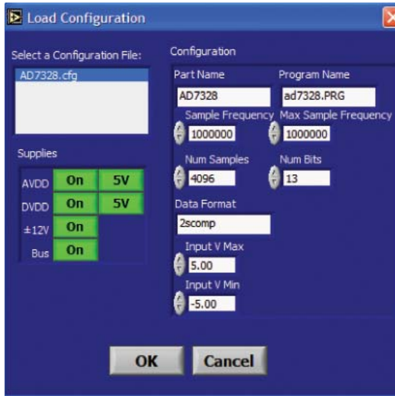
Figure 4. AD7328 Evaluation Software, Load Configuration Dialog Box
